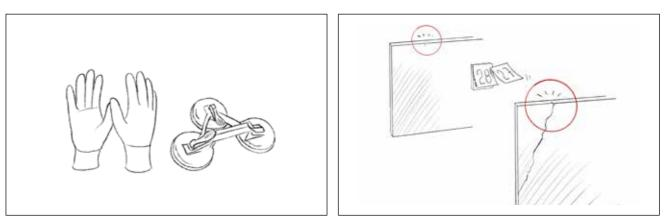
H andle the sheets with the utmost care and wearing clean gloves. Larger and heavier slabs must be handled with suitable equipment (suction cups). T he sheets must be stored vertically in areas sheltered from the sun and bad weather, away from heat sources, at a temperature between + 5 ° C and 35 ° C, with a relative humidity of less than 70%. Prolonged contact between Dècora Glass sheets and vulcanized black rubber is not recommended.
