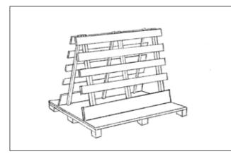
For safe transport and storage, use glass racks compliant with EC directives, taking care to fix them in order to avoid pressure on the windows. Follow the maximum load instructions on the labels of each truck.
