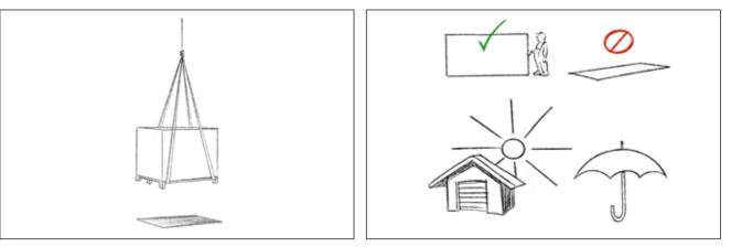
I t is possible to lift and handle the packages with a crane if properly harnessed. The harness must be made in a balanced way, so as to distribute the weight of the case evenly.
