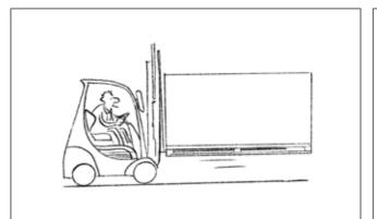
I t is possible to handle the packaging with a forklift, as long as it is equipped with forks with an adequate extension, in order to avoid instability phenomena and transport the packaging in safe conditions.
