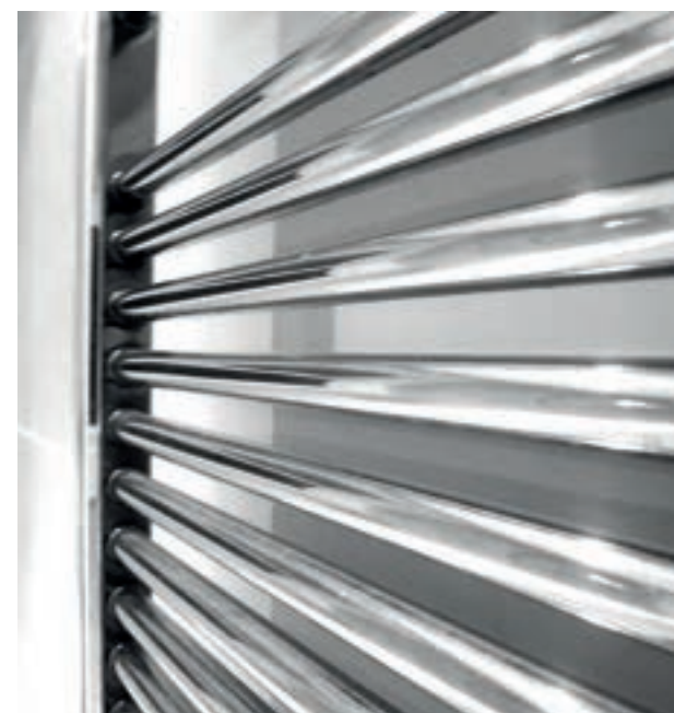
CC Tappings are 40mm less than the rail width and approx. 70mm from wall. We recommend using Hugo2 in a closed system incorporating an anti-corrosion inhibitor. All heat outputs based on Delta \Delta t 60°C.
