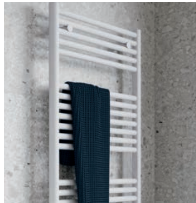
CC Tappings are 40mm less than the rail width and approx. 70mm from wall. We recommend using Hugo2 in a closed system incorporating an anti-corrosion inhibitor. All heat outputs based on Delta \Delta t 60°C.
